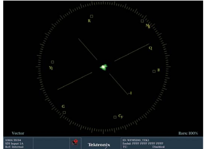
Figure 18. This Vectorscope is of a balanced Chip Chart. Note how close the entire trace is to the center of the vectorscope.
