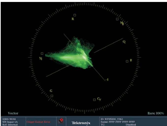
Figure 19. This is a Vectorscope of a typical image. An interview set in a backyard. The trace shows the red of the skin tones and the yellow/green of the grass and a bit of the blue sky.
