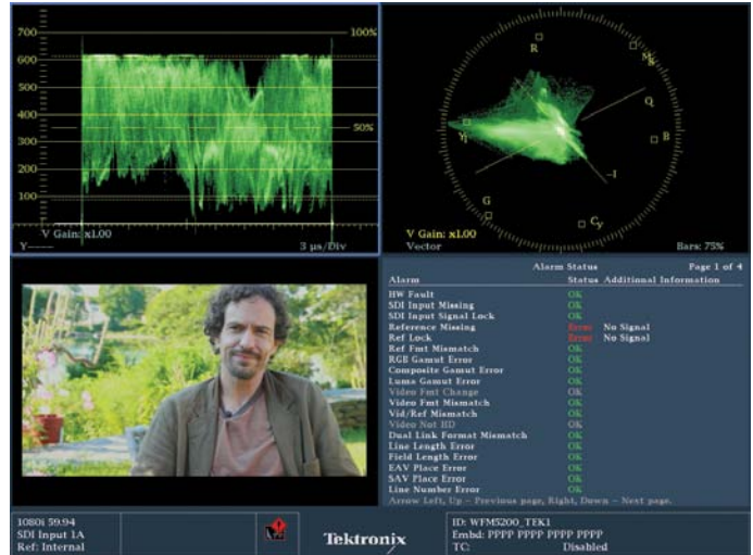
Figure 4. The Tektronix Waveform Monitor shows that the image doesn't take advantage of the full dynamic range. Blacks are lifted (above 0) and whites aren't at 100% (or 700 mv).
