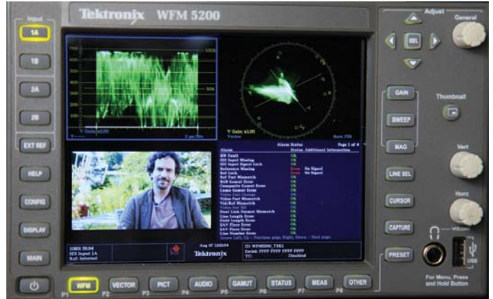
Figure 2. Tektronix WFM5200 is ideal for both color correction in a post production environment and for field production.
