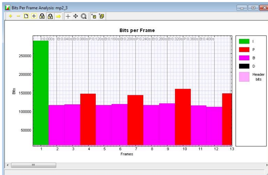
Figure 34: Bits per Frame Analysis graph – MPEG-2 example of Frame units display
