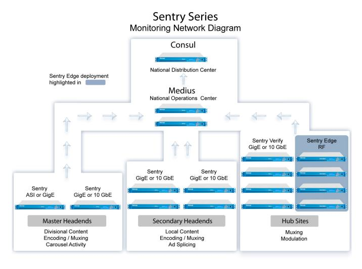
Figure 414: Sentry monitoring network diagram
