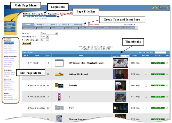
**Figure 4: Sentry Interface Components**
