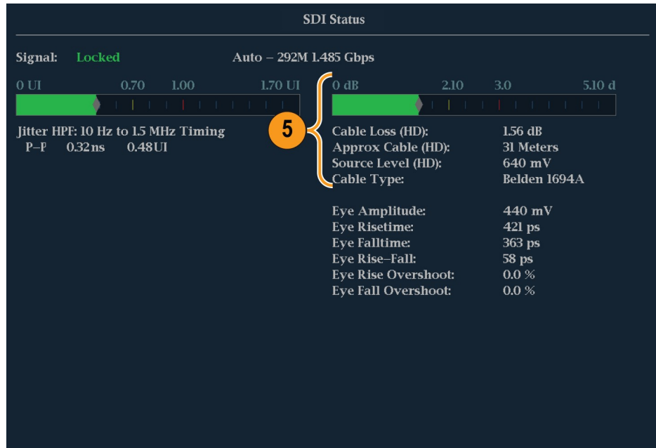
Figure 60: Cable loss information in the SDI Status display
