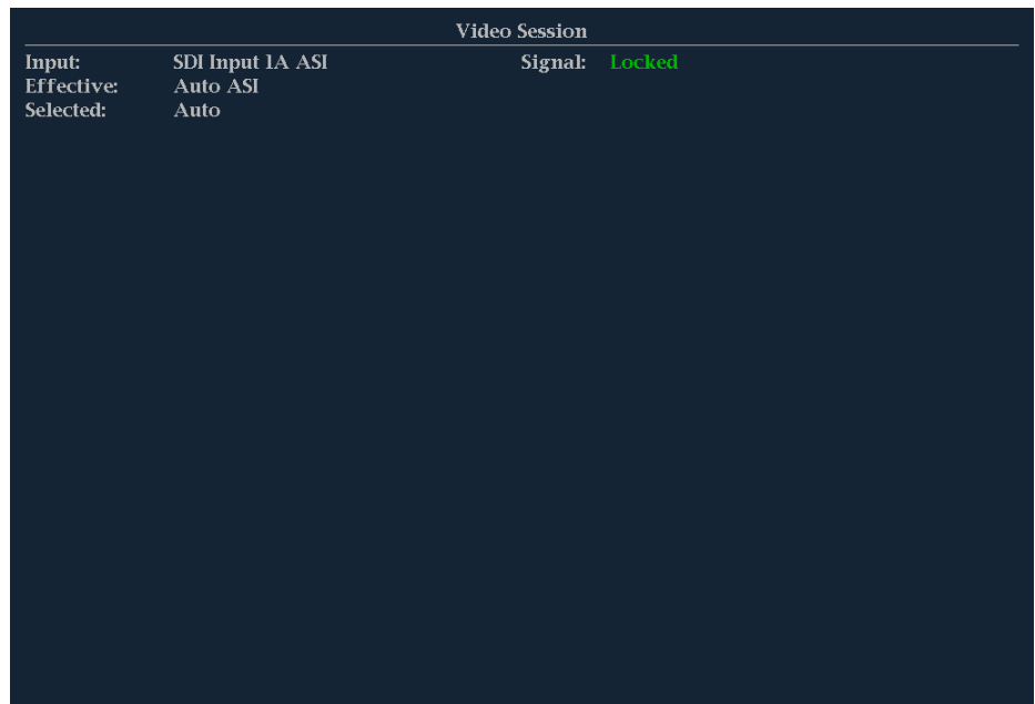
Figure 46: Video Session display of an ASI transport stream (WFM2300 Option ASI only)
