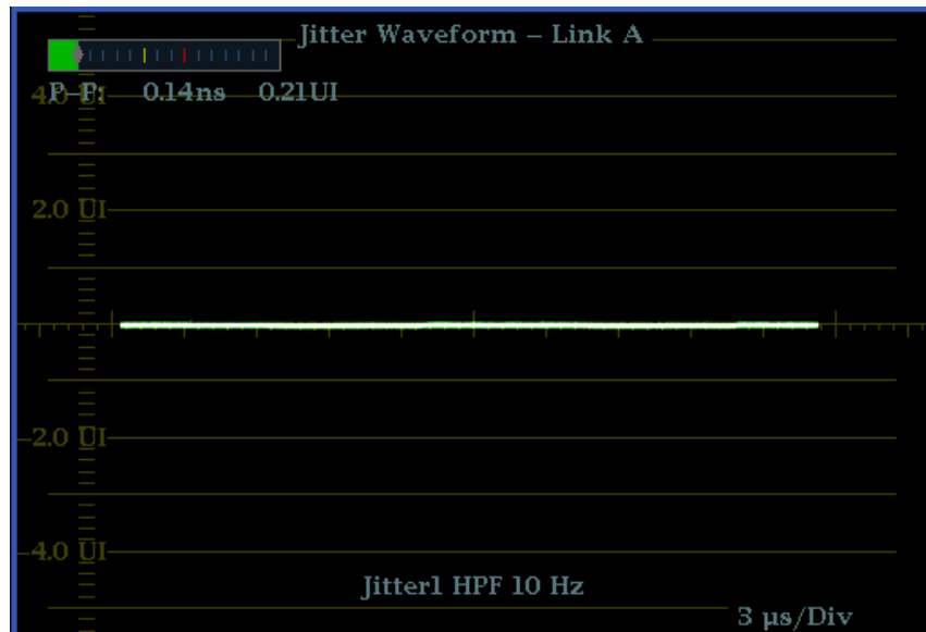
Figure 26: The Jitter display parameters as shown in a single tile when the instrument is in 4-tile mode
