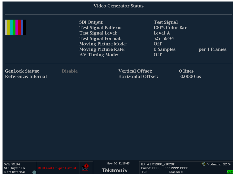
Figure 51: Video Generator Status display
