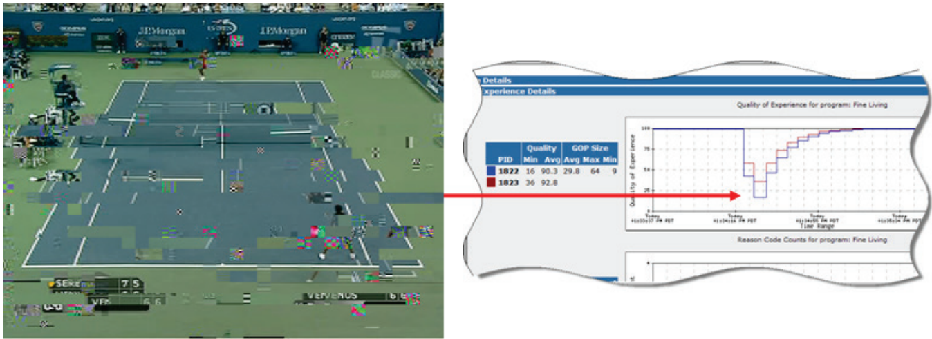
Figure 3. Example of how Video QoE score (in blue) gets reduced to indicate dissatisfaction.
